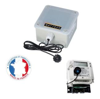
The Class A LoRaWAN® Flash'O from WATTECO is a long range, low power consumption, high performance and high quality sensor. It operates with any commercial electronic meter products equipped with a LED flash and provides connection to any wireless network using the LoRaWAN® protocol.
